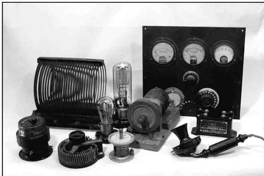
K2TQN’s early transmitter parts. From the left: a filament transformer; an oscillation transformer (coil); a 50-W filament rheostat; a 5-W 202 tube and socket; a 50-W 203 tube and socket; a blocking condenser; a rotary chopper, an old tube transmitter panel with various meters; an early microphone; and a magnetic modulator.
