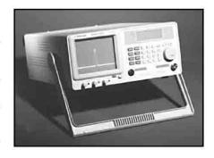
tions. A four-line LCD provides easy to read instrument settings and measurement values.
