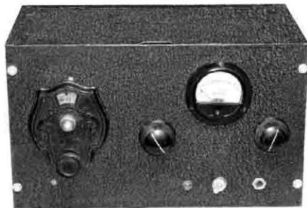
Front view of the 6L6/807 transmitter from an article in a 1949 issue of QST .
