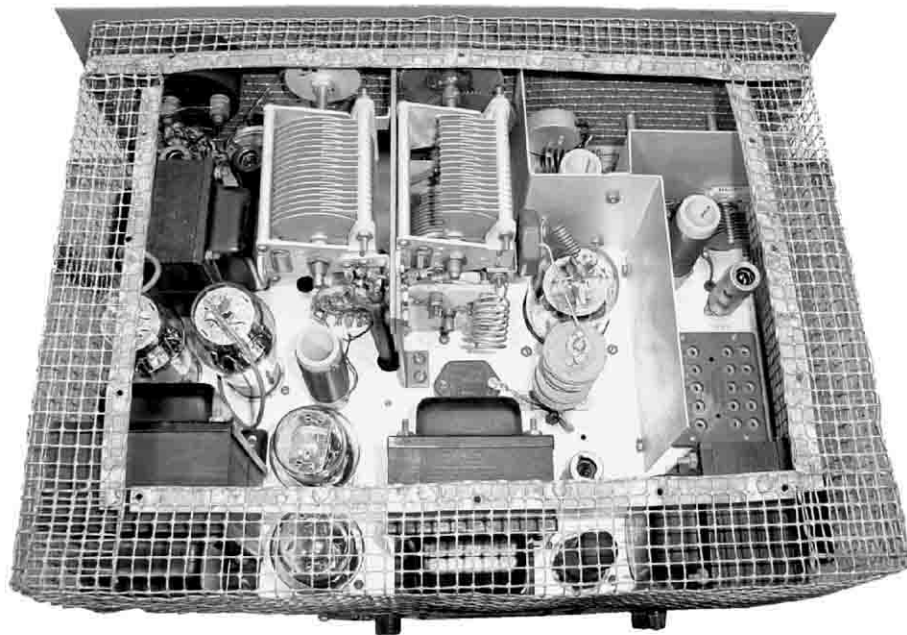
Viking I TVI shielding with the top cover removed.
