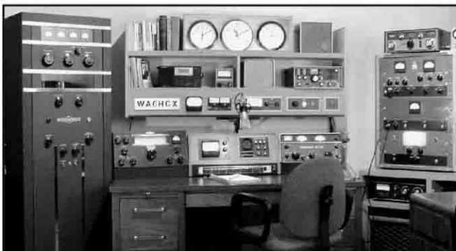
George Silva, WA6HCX. The transmitter on the left is a Collins 30K1, vintage 1947. It was the first big amateur transmitter built by Collins after the war. The final is a 4-125 modulated by a pair of 75TH's. Frequency bands are 80-10 with an AM output of 250 W. On the desk next to it is the 310B3 matching exciter/vfo. George built the console and cabinetry out of walnut. The receiver is a Hammarlund HQ200. The transmitter on the right is a Globe King 500B, which he uses on 160 meters. For several years now, George has operated almost exclusively on AM.
