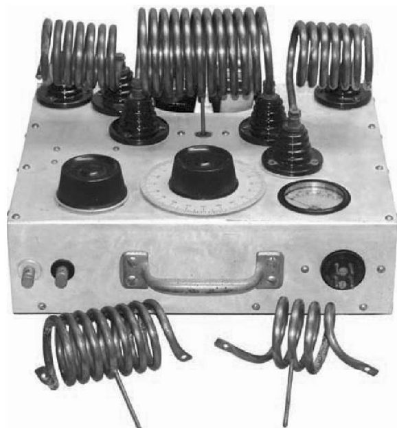
Front view showing the 80 meter coil mounted in the center, the two antenna coupling coils on each end. In the front are the extra 40 and 20 meter coils. From the left on the front edge are the key connections, the carry handle, and the 4-pin power connector. The controls from the left are antenna tuning and the plate tuning controls. The meter is a 0-100 milliammeter.
