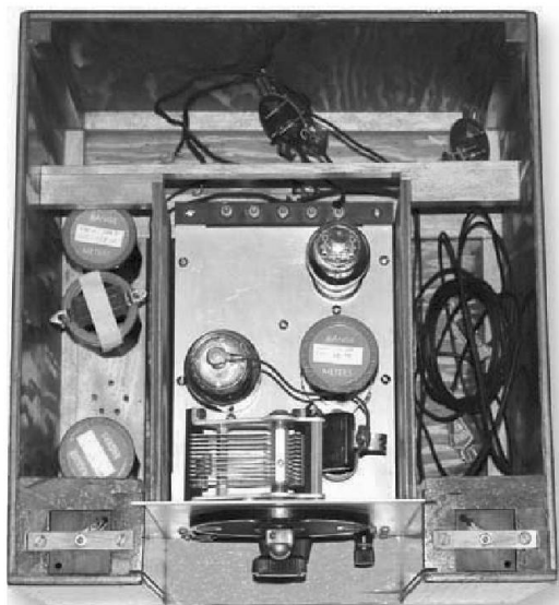
Receiver top view showing battery and storage compartments.
