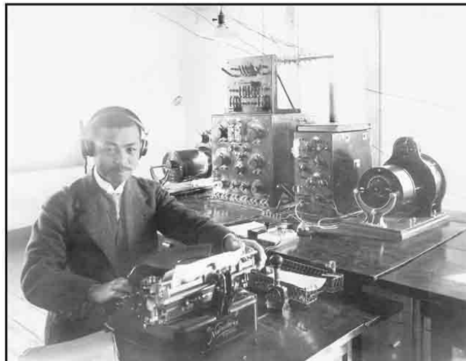
Figure 14—Sitting at his "mill," Superintendent Yonemura is ready to copy the next message at the Tomioka Receiving Station, call letters "JAA." Note the early tubes on the panels of the two receivers. The cylindrical units at either end of the receivers are called Loose Couplers. They have tapped and movable coils, and are used to help tune in stations. The antenna selector switches are on the panel above the receivers. There is a single light bulb overhead. His logbook is on top of the receiver on the right. (Photo 1921)
