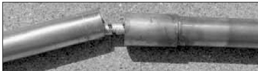
Figure 4—The bungee cord runs through each of the antenna elements.
