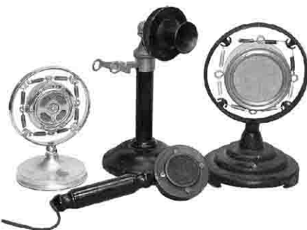
Figure 2—Two examples of a suspension microphone, a Shure 5B on the left and the Amplion GM on the right. The taller one is an old "Conn Tel & Elec Co" telephone converted into a mike, and the hand mike is an Amplion MH from the late 1920s or early 1930s.
