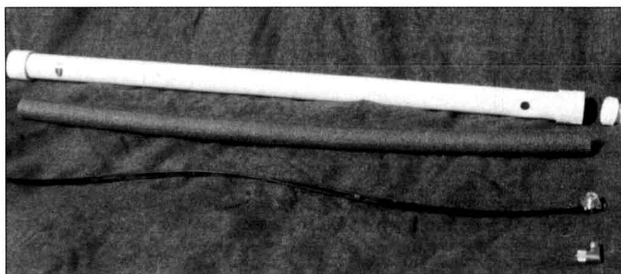
The disassembled J-pole antenna. The twinlead antenna core is shown at the bottom with the M359 right angle connector removed. It's placed within a foam insert (middle) which keeps the antenna centered within the PVC tube (top). This is the construction technique used by the JADE Products "JADE-POLE" antenna.
