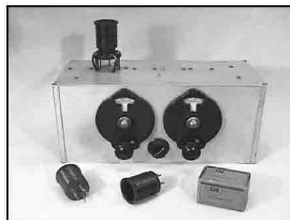
The Silver-Marshall "Round the World" Four. The left-hand vernier dial controls the tuning, the right-hand vernier dial controls regeneration. The small lower knob regulates the detector filament voltage and at the extreme anti-clockwise position turns the entire set off. Four different plug-in coils cover from 17.4 to 204 meters.
